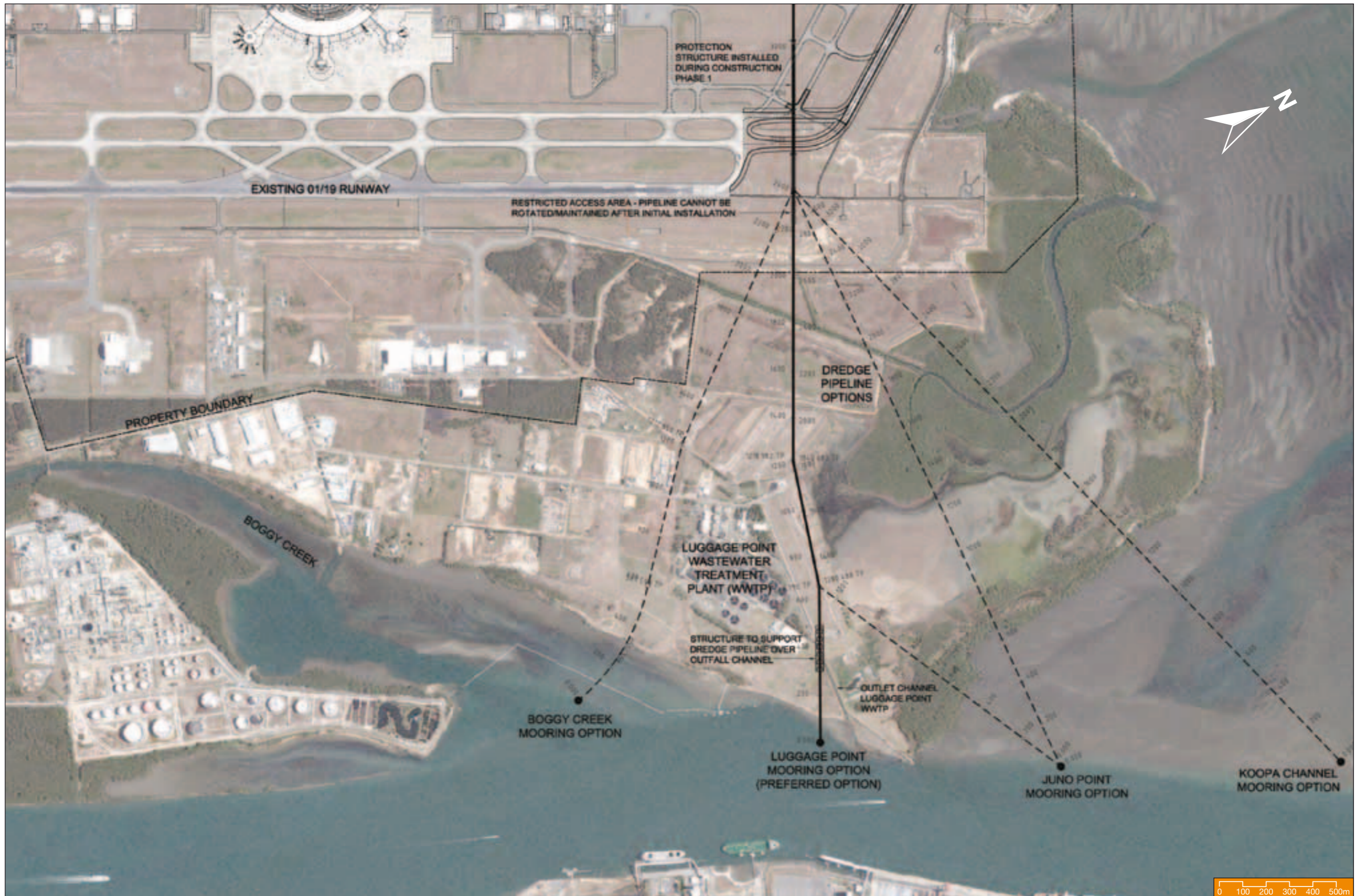
Figure 4.21: Dredge Mooring Location and Pipeline Routes.
